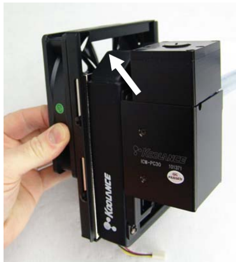
Slide radiator/pump to desired height and retighten 4 bracket screws
