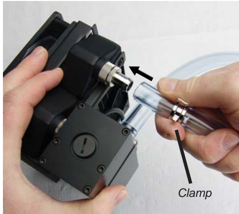
Push unattached tubing onto radiator barb
