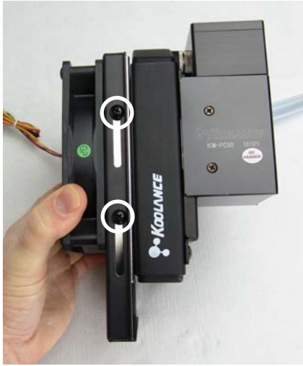
Loosen bracket screws (2 per side)
