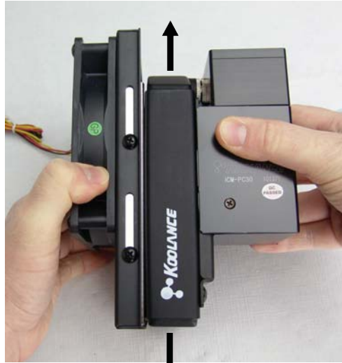
Slide radiator/pump to desired height and retighten 4 bracket screws
