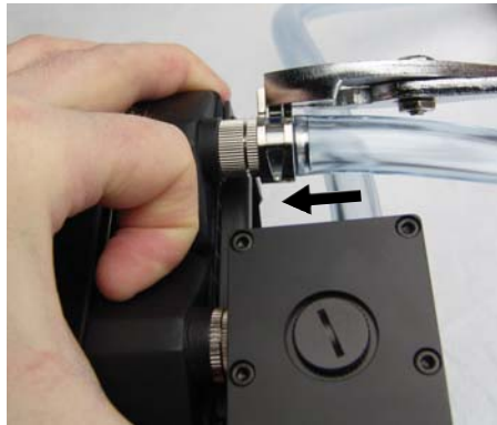
Move clamp onto radiator barb
