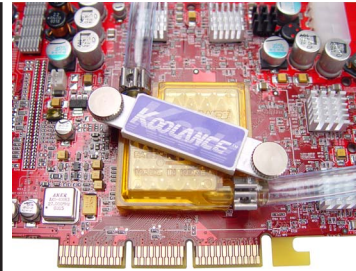
(Chipset Cooler mounted on an ATI Radeon 9800 Pro)
